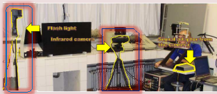
Figure 4. Laboratory set up for the pupillometry study conducted under artificial lighting.
